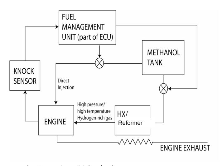
Low temperature catalytic reforming CH<sub>3</sub>0H → 2H<sub>2</sub> + CO (syngas) Endothermic decomposition Syngas has more energy than methanol
