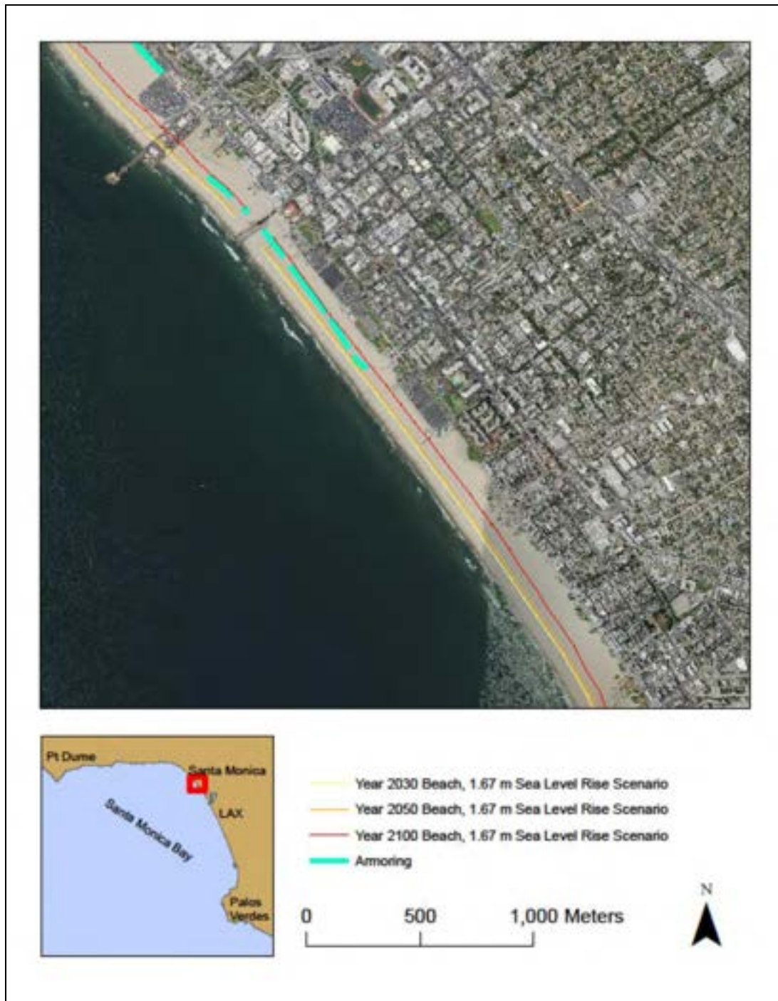
Figure 11. Shoreline retreat from sea level rise by 2030, 2050, and 2100 for the 1.67 m scenario in the Santa Monica Pier vicinity.
