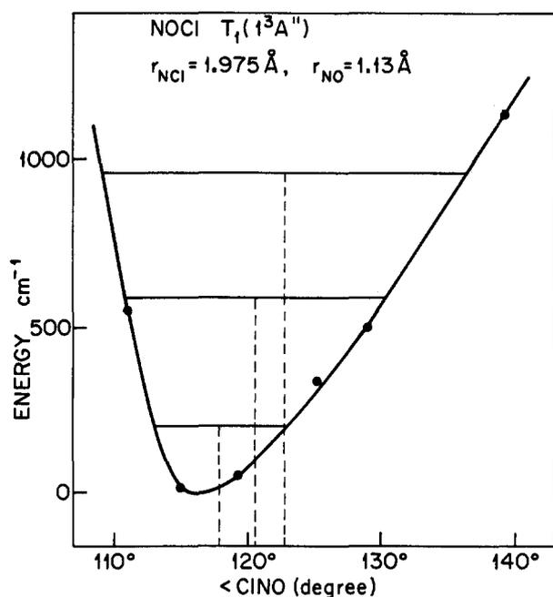
FIG. 7. The NOCI bending potential obtained in the *ab initio* CI calculations (Ref. 2) for  $r_{\text{NO}} = 1.13 \text{ \AA}$ , and  $r_{\text{NCl}} = 1.975 \text{ \AA}$ . The dashed lines show the center angle for each bending level. The center of the wave function does not necessarily coincide with this value, and is probably further shifted to the right due to the asymmetry in the wave function.
