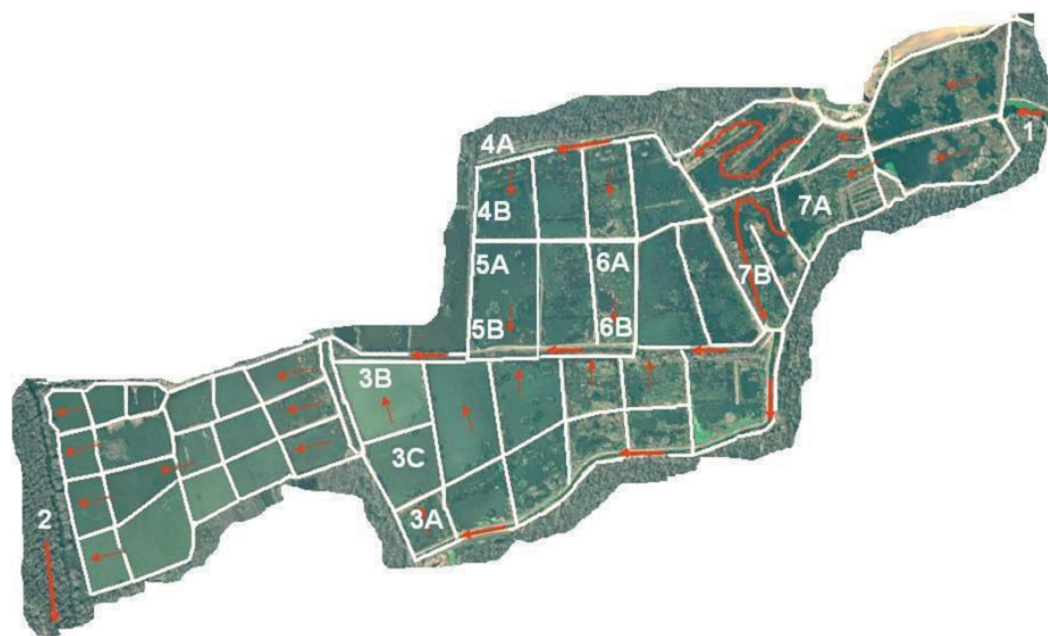
Figure 1 Prado wetlands showing the sampling sights for June–November 2004. The arrows indicate the direction of flow. The wetlands treat 50% of Santa Ana River water. The sampling sites were chosen based on their percentage of plant cover: (1) inflow; (2) outflow; (3) 25% cover; (4) 50% cover; (5) 75% cover; (6) 50% cover; (7) 100% cover. Letters A and B after the numbers indicate influent water to that cell and effluent water out of the cell as seen by the direction of water flow. Two cells were used for each treatment.
