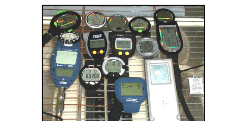
Figure 4: Dive computers in water bath used for tests.
