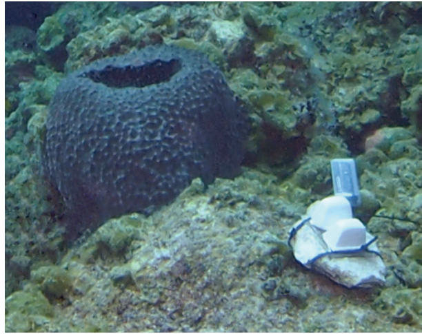
Figure 3. Plaster of Paris bricks (bottom, right) with temperature and relative light level data logger (Onset Computer Corp.) placed next to a barrel sponge by divers at Eleuthera Island, Bahamas. Photo: David Ginsburg.
