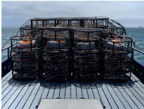
Figure 3. Pop-up Gear. Note: Pop-up gear being tested on a fishing vessel during the Spring 2025 fishing trials. The line and buoy are stored with the crab pot (Chadwick & Mullins 2025).
