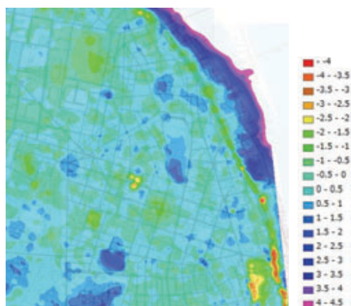
Fig.6 Difference of DEM (2005 and 1950) [Source: Yonezawa 2009] Map (1:2,000) overlaid with difference of DEM. The darker-shaded area is lower in 2005 than 1950.
