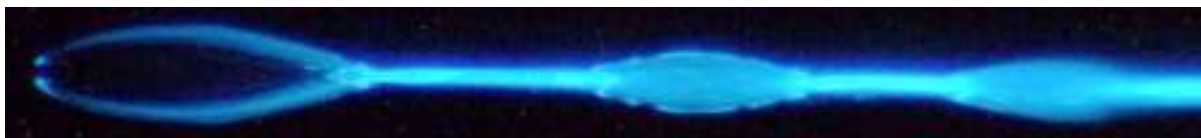
Fig.1 A flatjet generated by the impingement of two microjets, one containing a luminol + copper sulfate solution and the other composed of highly concentrated hydrogen peroxide solution. The flow direction was downwards, but the figure was tilted such that the flow here is shown from left to right, and the original microjets are at the plane perpendicular to the paper. The characteristic blue chemiluminescence of luminol is seen where the two liquids mix efficiently. The most important aspect here is that the first flat part of the jet (the first leaf ) is mostly dark, with a faint glow appearing at its end, highlighting that a well-defined liquid–liquid interface is created there. We have demonstrated that the liquids only mix in this region due to diffusion through the interface [1].
