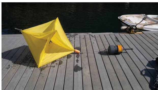
Figure 4. The RESL drifter. One of our three drifters when it is completely assembled. Each drifter system is composed of a drogue, a tether, and a surface float with a radio antenna.
