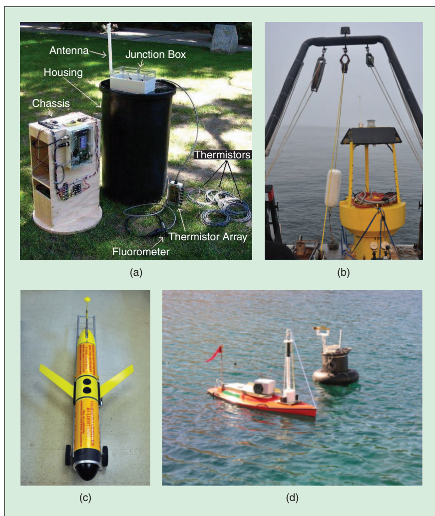
Figure 1. Deployed marine sensors. (a) Marina buoy components, (b) coastal mooring, (c) Webb Slocum autonomous glider, and (d) ASV and deployed marina buoy.
