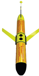
Fig. 1. HeHaPe, one of two USC Slocum gliders.
