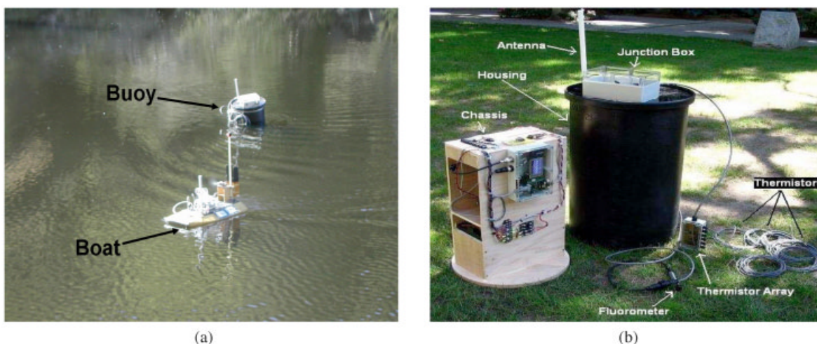
Figure 4. NAMOS components. (a) System of buoy and boat deployed during the campaign. (b) Detailed system description of a buoy.
