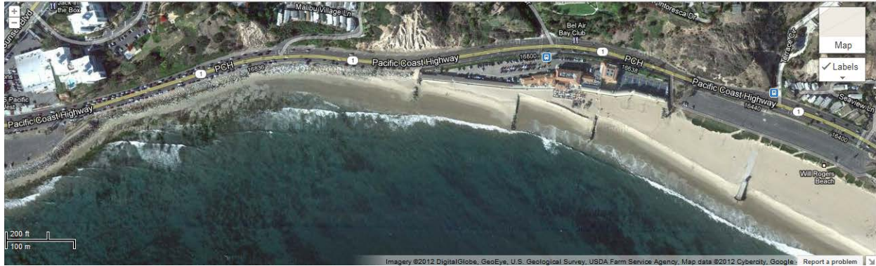
FIGURE 6: BREAKWATERS BUILT ALONG THE SHORELINE TO PREVENT EROSION OF THE DESIRABLE WILL ROGERS BEACH IN PACIFIC PALISADES. THE PACIFIC COAST HIGHWAY IS THE ONLY EVACUATION ROUTE FOR SOME COASTAL RESIDENTS FROM THESE SHORELINE AREAS (HIGHWAY HIGHLIGHTED IN YELLOW). SOURCE: GOOGLE MAPS
