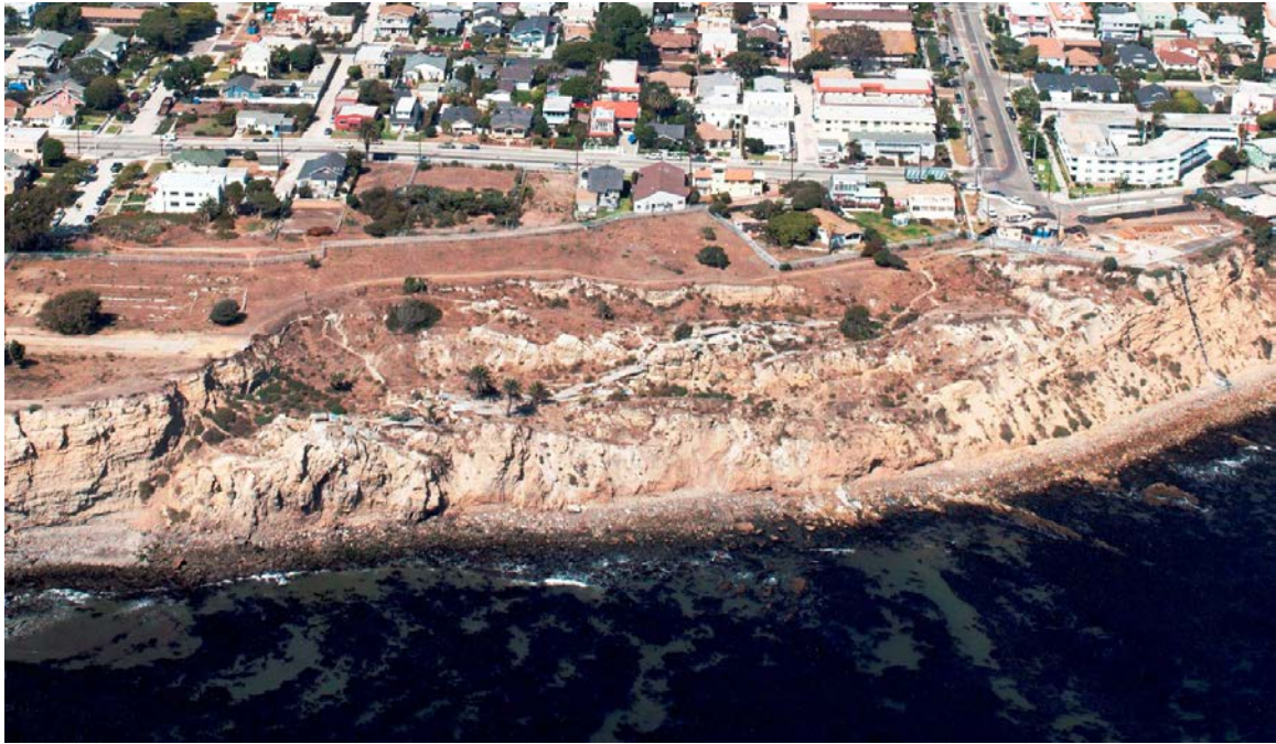
Figure 12. Landslides east of Point Fermin present geotechnical challenges in this segment (California Coastal Records Project Photo 201002554).
