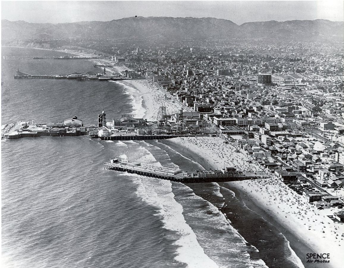
Figure 9. View north circa 1930 from Venice Beach with Sunset pier (removed circa 1940, foreground), old Venice pier (destroyed 1946), Ocean Park pier (removed late 1960s), Crystal pier (removed mid-1940s), and Santa Monica pier, the only one still standing. Note beach width stabilizing effects of the piers (Spence Air Photos, accessed from http://venicebeachbustours.com ).
