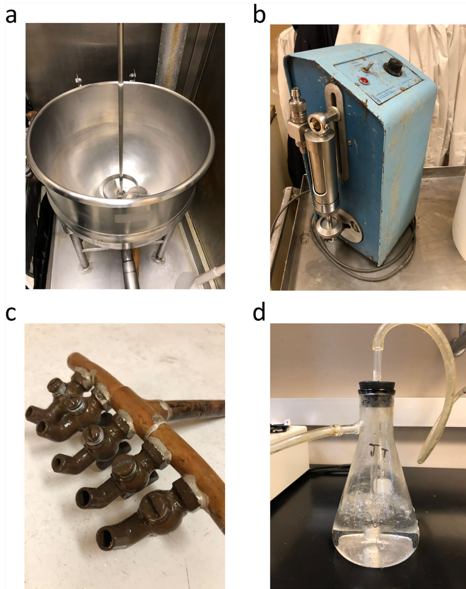
Figure 1. Equipment. (a) Steam-jacketed kettle. (b) Pump. (c) 5-headed nozzle. (d) Bubbler.
