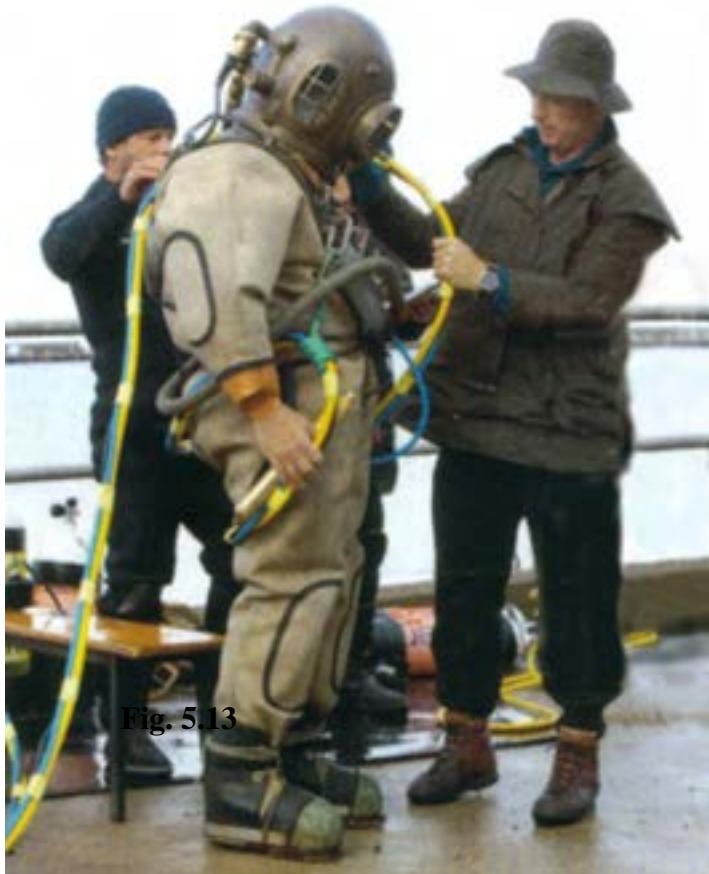
Fig. 5.16 A "hard hat" or standard dress rig.
