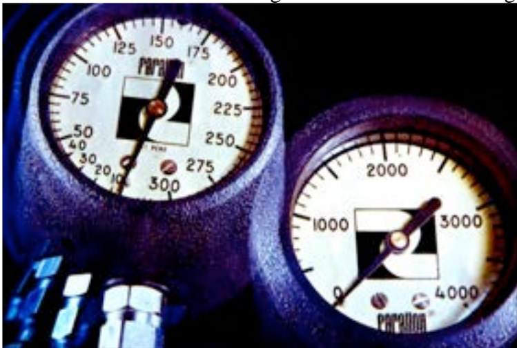
Fig. 5.21. Depth and contents gauges (calibrated in feet of sea water and psig, respectively).
